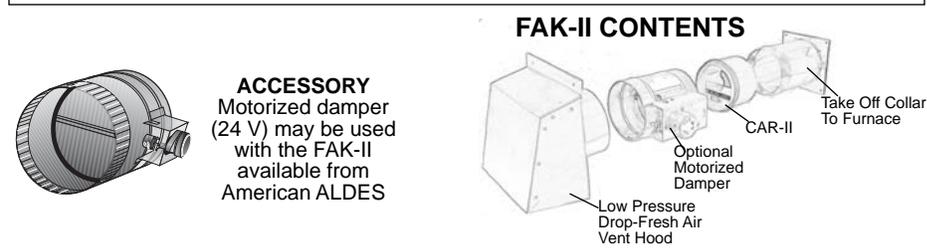
Mark and cut out a circular opening matching the diameter of the takeoff provided in the kit in the return ducting to the air handler. **DO NOT CUT INTO THE HOUSING OF THE FURNACE**, as this will void the warranty of the furnace.
